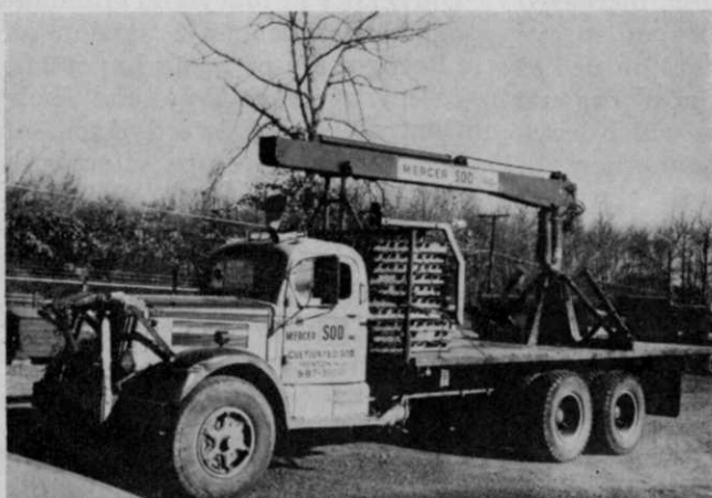
Outfitting all trucks with boom loaders (left) has expedited shipments, reduced cost of unloading palletized sod.
