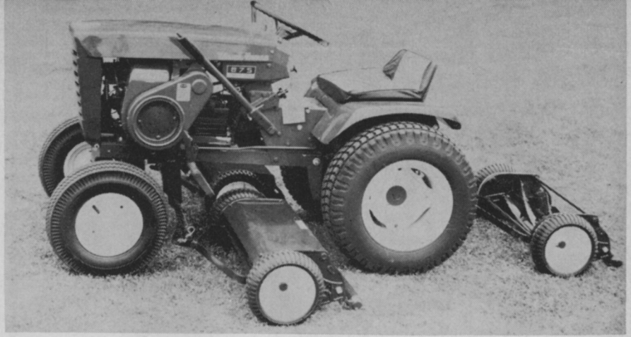
Roxy Mower Model UM21-3W has been approved for all Wheel Horse Standard Chassis Tractors, including 1966 models, Roxy-Bonner announces. The three gang mount cuts a 58 inch swath and reportedly keeps wheel tracks to a minimum. Other models of the mower are available for various lawn and garden tractors. Drags cutting 60 to 96 inches, and 50%-heavier drags for 72 to 132 inch swaths are also produced. Roxy-Bonner, Inc., 2000 Pioneer Road, Huntingdon Valley, Pa. 19006 has details.
