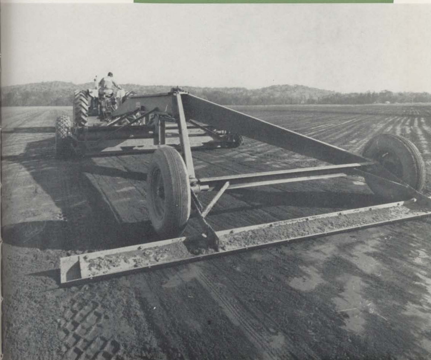
A hydraulic land leveler prepares a new field at Summit Hall's Potomac Valley Turf Farm. This field is part of the more than 1000-acre farm under development in southwestern Maryland. Story on pg. 27.
