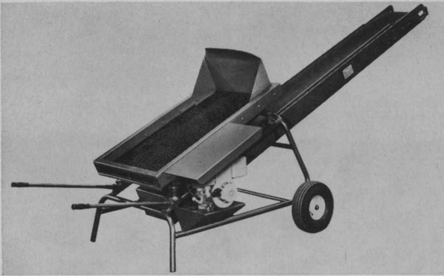
Single power source on the Royer Powerscreen 42 actuates the screen deck to sift soil, and hooks up with a conveyor belt which can be elevated to discharge height convenient for loading or stockpiling.
