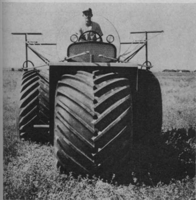
Goodyear "Terra-Tires" give the "Big-A" spreader no-sink traction to prevent erosion due to tire ruts.
