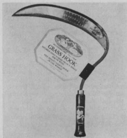
Rugged grass hook is hand forged and shaped by eye from a single bar of steel. Blade is 1 3/4 inches wide and has an 11 1/2 inch cutting edge. For more information write to Witherby Products Div., John H. Graham & Co., Inc., 105 Duane St., New York, N. Y. 10008.
