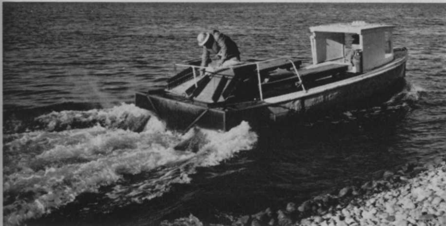
Seattle designed and built simple, efficient equipment for distributing copper sulfate by power launch.
