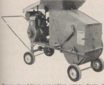
Kemp shredding capacities range from 4 cu. yds. up to 101 cu. yds. an hour. Kemp model 8-OX above, shreds 12 cu. yds. an hour.
