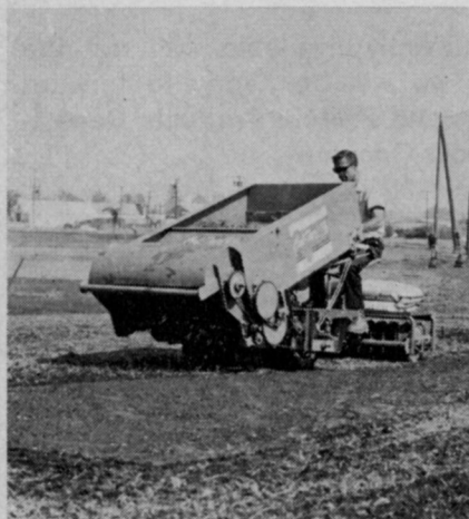
Small area planter automatically distributes and presses bermuda stolons into soil and plants half acre per hour. Capacity is 10 bushels.
