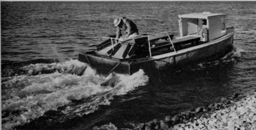
Seattle designed and built simple, efficient equipment for distributing copper sulfate by power launch.
