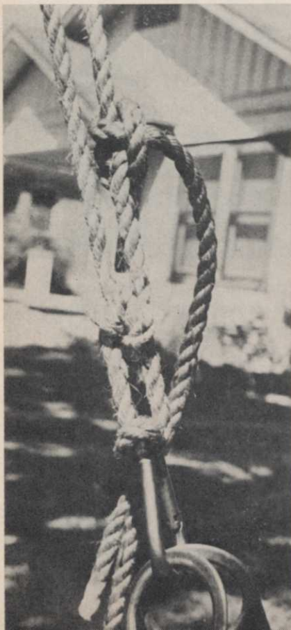
Fig. 1. (left) Safety rope fastened to the snap on the tree surgeon's saddle. A round turn is made in the eye of the snap, and is secured with a bowline knot. The upper knot on the right is the climber's sliding hitch knot.
