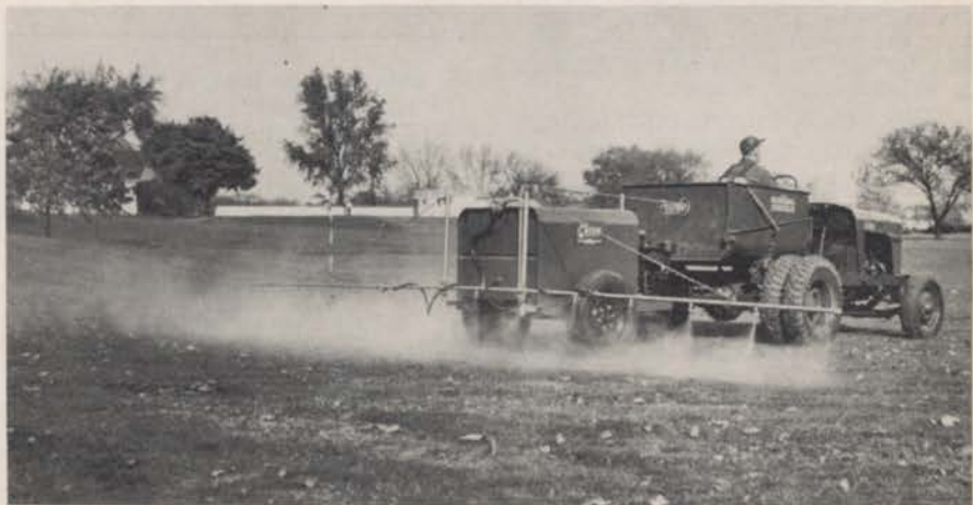
With nozzles set to spray at 65 degrees, this boom spray system delivers even coverage with little drifting caused by wind. Boom is 22 inches from the ground.
