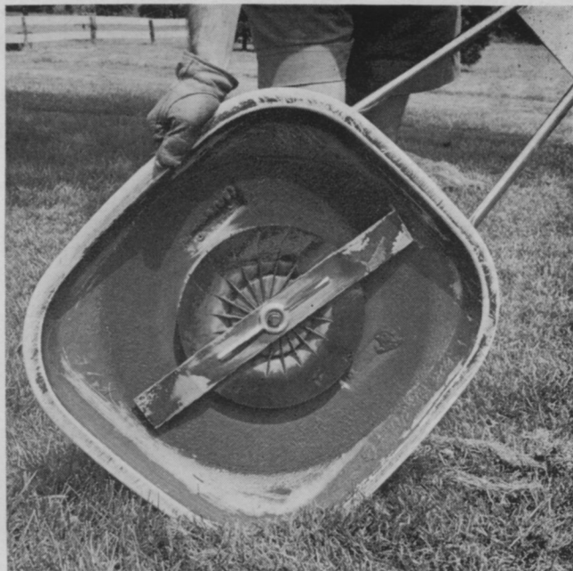
Design of air cushion mower is simplicity itself. Note the rotor, that throws out a curtain of air, is deflected downward by housing. In the calm center is the rotary cutting blade, activated by the same driveshaft.
