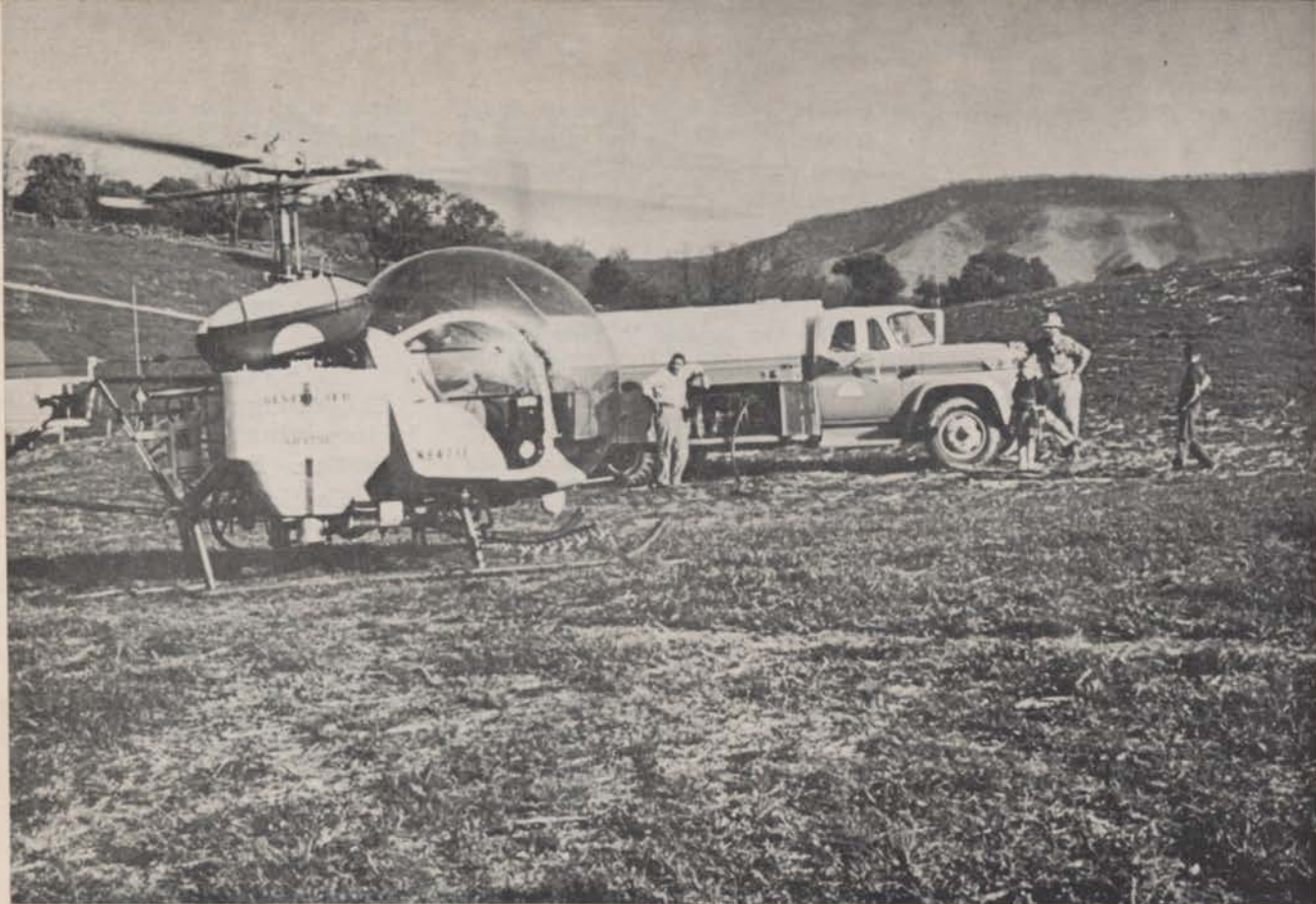
Equipped for pastureland spraying, helicopter tanks are loaded with herbicide from companion service truck.
