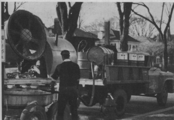
Mist blower being filled with AMOCO Elm Spray, to control Dutch elm disease on city parkway.
