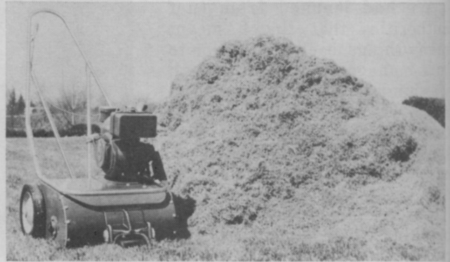
Thatch-O-Matic Model PR-6316 (left), from Parker Sweeper Co., has 104 rotating and self-cleaning tines and is powered by a 3 h.p. engine with a centrifugal clutch and recoil starter. Tine reel runs at 1200 R.P.M. or 125,000 tine-contacts per minute. Tines are said to be designed to comb out debris without mutilating the sod. Pictured below is a huge pile of thatch raked from sod with this Thatch-O-Matic.
