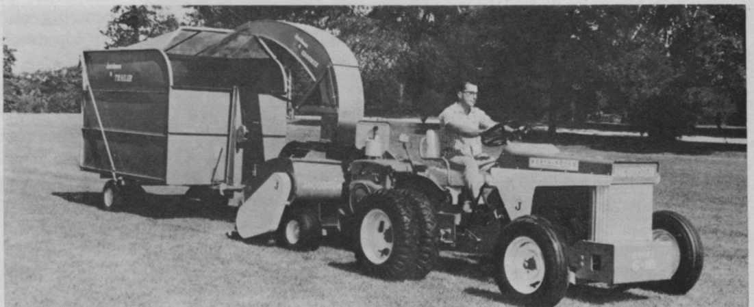
Turf Groomer pulled by a vehicle blows waste into trailing bin. Trailer is 11\frac{1}{2} ft. long, 5\frac{1}{2} ft. wide, and 8 ft. high, and is equipped with a rear release door and a winched draw bar for easy dumping of collected thatch.
