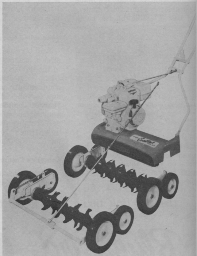
Contour Thin-Cut Renovator , Model 18, made by Henderson Manufacturing Co., cuts 18" vertically to the ground line, removing thatch and other undesirable material without harm to soil. Powered by either 3 or 4 h.p. Briggs & Stratton engine. Fifteen double-end steel blades cut grasses up and away from the operator for extra safety. Interchangeable Cyclo-Safe cutter unit (shown under housing) converts unit to a lawn mower.
