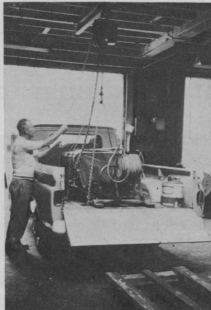
**Five minutes** is enough time to switch sprayers. Dolly (lower right) carries rig to or from the truck. Four bolts secure the skid to the truck. One man can perform this time-saving operation, cutting down on man-hours.
