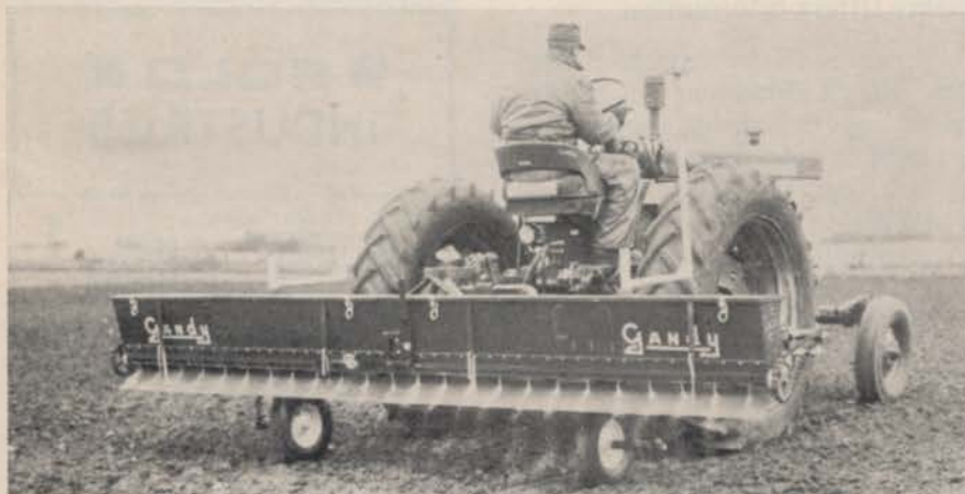
A granular chemical applicator said to apply as little as 5 pounds material per acre is manufactured by the Gandy Co., Owatonna, Minn. The applicator is made in 4 sizes from 8 to 14 ft.
