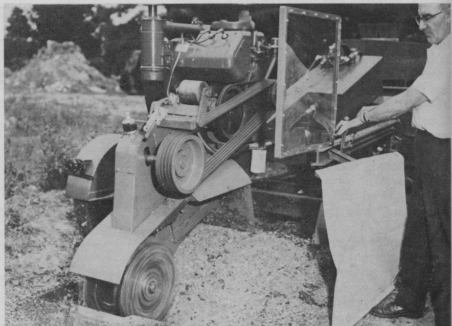
Troublesome stump in foreground was delaying landscape job until Stump-King came along. Makers of this new machine say it is ready to begin cutting as soon as it's backed up to a stump; no need to reposition unit's wheels. Blade is lever-controlled.
