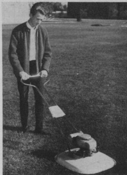
From the large display of equipment and supplies demonstrated at the 11th annual Rocky Mountain Regional Turfgrass Conference, this lawn mower drew attention because it employs a unique vacuum operating principle. The rotary mower has no wheels, propels itself by "floating" one-quarter inch above the surface. Jerry Nelson, CSU junior in landscape design, demonstrates.
