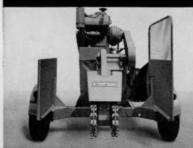
Fixed travelling wheels need no adjustment before starting the cutting operation. Back up to stump and start cutting.
