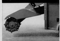
Cutter head, with 30" forward travel, reaches out for hard-to-get-at stumps. Low boom gives extra overhead clearance.
