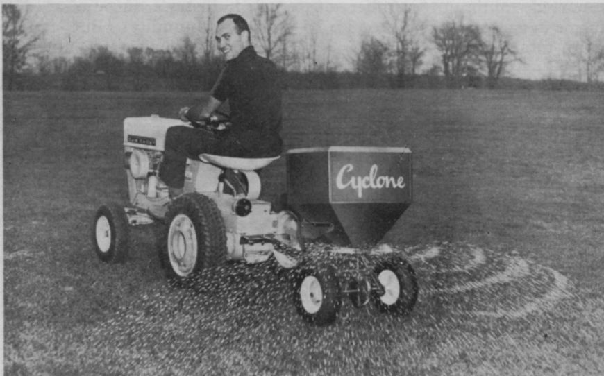
This Cyclone Model 99 is a new pull-type broadcast spreader/seedler designed to spread fertilizer, seed, and other materials without stripes and double overlaps. Cyclone makes a manual model also.
