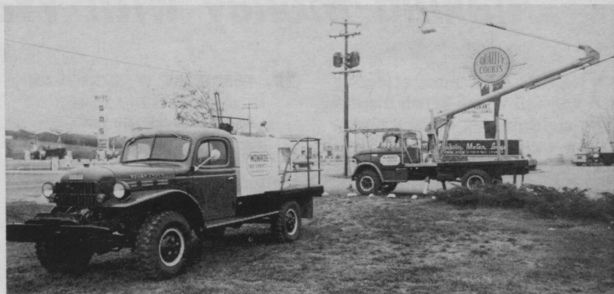
A Dodge Power Wagon with tank, pump, hose, and a guardrailed rear platform is heavy-duty equipment for roadside spraying. In the background is a hydraulic Skyworker for utility line maintenance.
