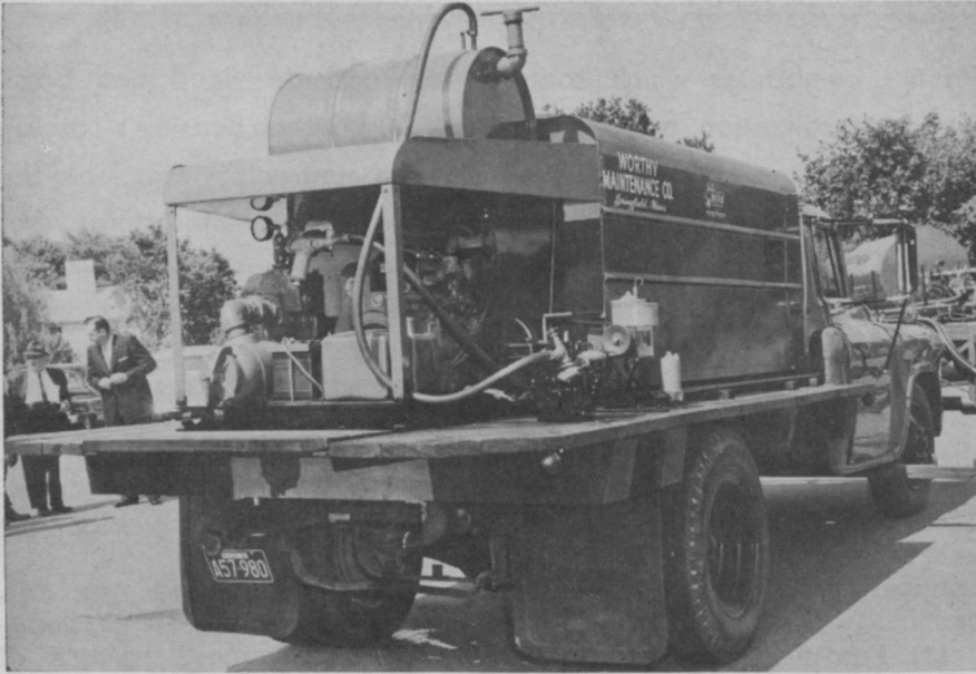
Rear view of this spray rig operated by Worthy Maintenance of Springfield, Mass., reveals the complexity of pumps, tanks, hoses, and other quality equipment necessary for competent contractual work for highway roadside spraying.
