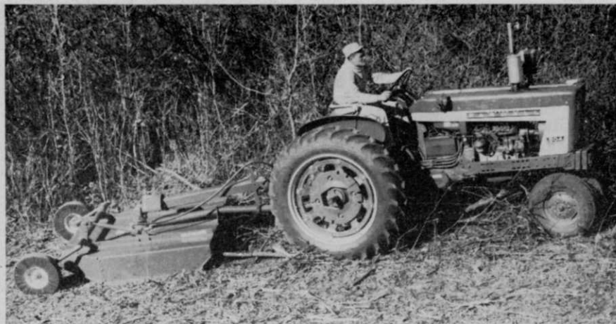
Whirling cleaver action of the heavy-duty 410 Rotary Cutter completely splinters thick brush, trees, and growth that can be bowled over by the tractor equipped with front bumper bar, McCormick International reports. Cleavers are pivot mounted and free swinging.
