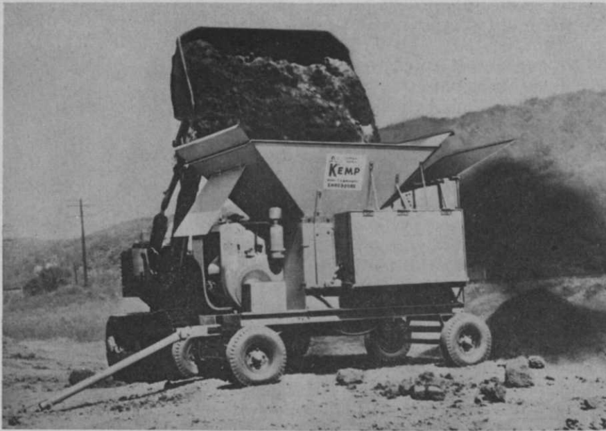
The New No. 101 "King Kemp" shreds up to 101 cubic yards of wet or dry soil an hour. Kemp shredders are used for topsoil, bedding, litter, mulch, and other materials requiring quick, uniform shredding, grinding or pulverizing.
