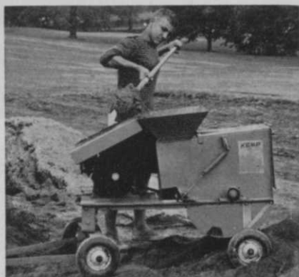
No. 8-0 Work Horse, shreds and aerates 4- to 12-cubic yards an hour.
