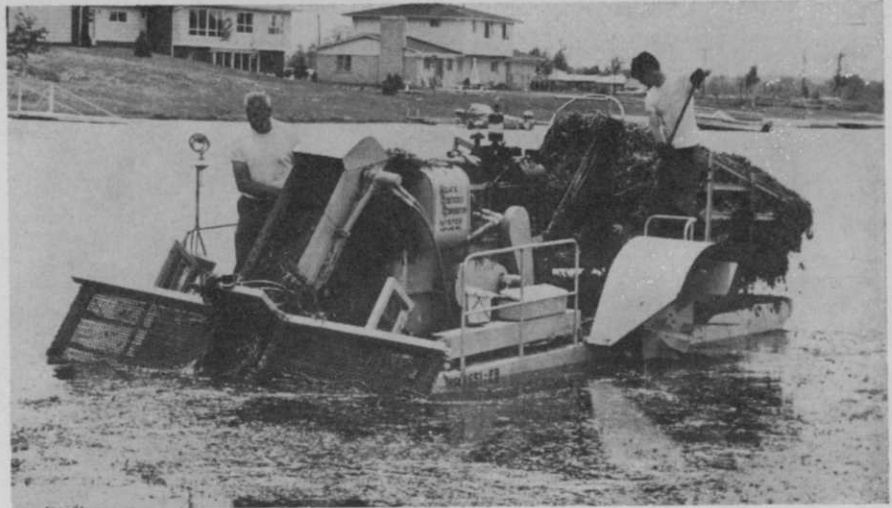
Aquatic Harvester is said to control water weeds in lakes, streams, and canals by cutting submerged weeds up to a depth of 5½ ft., and depositing them in a service barge. Machine, manufactured by the Aquatic Controls Corp. in Hartland, Wis., can harvest a full acre of weeds per hour, the firm claims.
