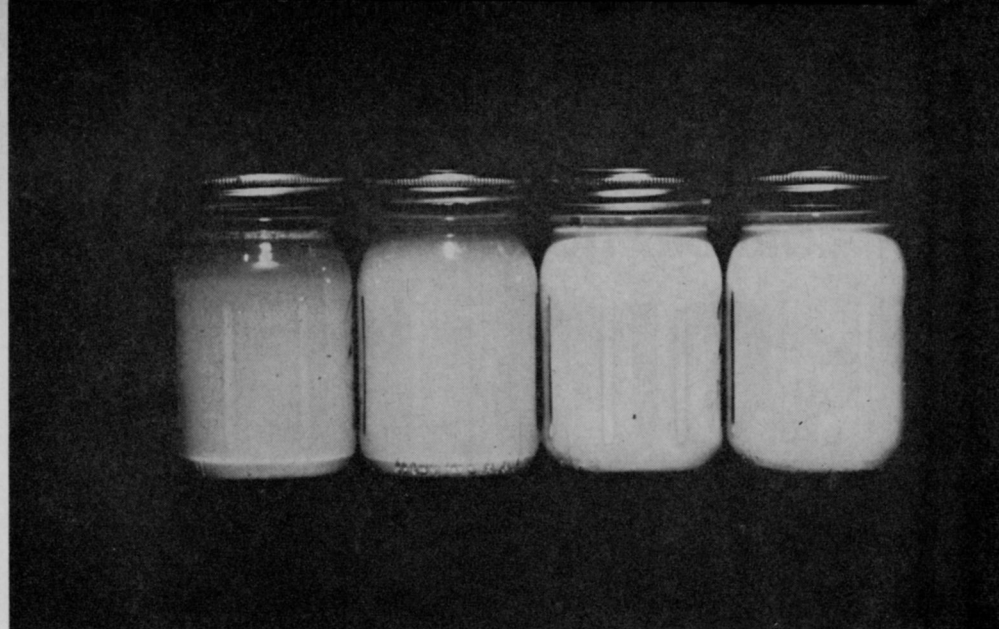
Here's a simple comparison test applicators can use to see if formulations measure up to necessary standards of quality. The two products on the left are much poorer emulsions than the two products on the right. Details for using this test are spelled out in the article.
