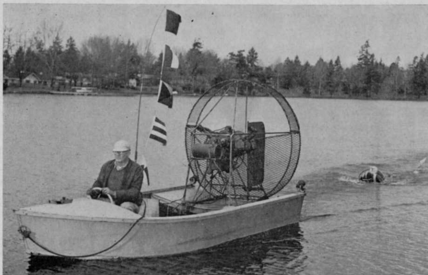
Submerging diver , left, rides diving plane toward lake bottom for look at weed infestation. Pilot George Harris (in airboat) is able to maneuver while towing the diver because the towline is attached to a special hitch in keel of boat under operator's chair. Above, diver Henry Carsner explains what he found to son Jim who is mapping the infestation.
