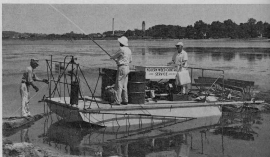
Typical of modern , custom-designed equipment used by aquatic weed control companies is this barge belonging to Modern Weed Control Service of Grand Rapids, Mich. Owner Vic Scholl is pleased with the Douglas Fir plywood device which is 8 feet long and 2 feet wide.
