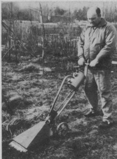
Sheen X500 flame gun, described by the distributor as a versatile machine which offers new and positive weed control and soil surface sterilization, is now being marketed by the Smrt Import Co., 1105 West Plainfield Rd., LaGrange, Ill. The English-made device features a heavy-duty pump, pressure gauge, and control valve, and can be hand held or operated on a wheeled chassis with a hinged hood. According to Smrt, the Sheen X500 permits continuous use over a large area and provides a steady, completely controllable flame. Applicators may write the company to obtain descriptive literature, prices, and a free booklet on flame gun usage.
