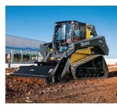
hinge pin of 11 feet allows for easy dumping into trucks and convenient transport of pallets of heavy pavers or other hefty materials. The cab offers clear sight lines to the bucket corners, above and below the lift arms and the jobsite both forward and backward. The 331G can be paired with more than 100 John Deere attachments to make the machine a versatile workhorse on any jobsite. Options include side lighting, rearview camera and onboard-grade indication among others.
