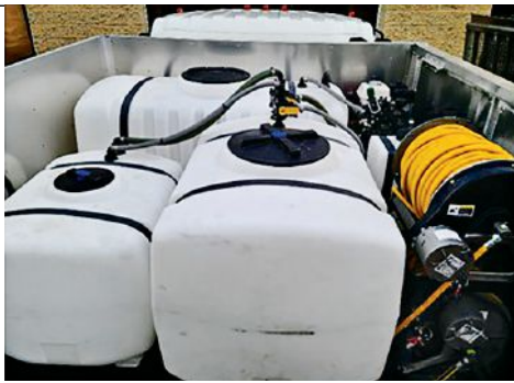
← THREE IN ONE Green Lawn Fertilizing's spray trucks are equipped with three tanks totaling 600 gallons of capacity.
