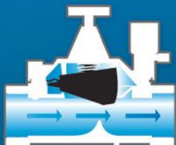
ULTRAFLOW® SERIES Straight-through flow path
