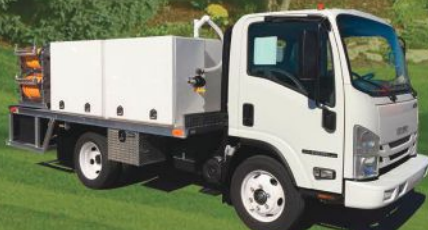
Isuzu NPR HD with Spray Rig 13' Bed & 600/200 Gallon Tanks 297 HP Gas Engine, Automatic Transmission, 14,500 lb. GVWR, 19.5 Tires, AM/FM CD Player, A/C, P/S, Power Windows & Locks, Tilt Wheel, (4) Boxes, 400' Hose, Hand Wash, Tow Pkg, (Other Options And GVW Ratings Available)
