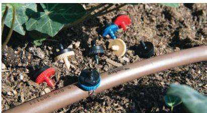
**Hunter** introduced a family of pressure-compensating drip emitters for its micro-irrigation line. Featuring flow options of up to 6 gph, they are available in three inlets: self-piercing barb, 10/32 thread and 1/2-in. female thread. The barb and 10/32 thread models are offered in .5, 1, 2, 4 and 6 gph models; the 1/2-in. female threaded model is available in 1 and 2 gph.
