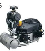
horsepower models. This family of products now encompasses 16 different engines ranging from 19 to 38 horsepower. The Kohler closed-loop EFI engines include an oxygen sensor that analyzes the air/fuel mixture in the muffler. If the oxygen level strays from the ideal air/fuel mixture, the sensor triggers adjustments to the amount of fuel injected into the system. The carburetor-free design of the EFI line can lead to fuel savings compared to comparable carbureted engines, the manufacturer says.
