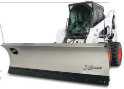
blade left or right. Available in 8- and 9-ft. widths, XBlade combines Fisher's exclusive X-bracing with corrosion-resistant, stainless-steel moldboards and proven trip-edge design. **Fisher** *II FisherPlays.com*
