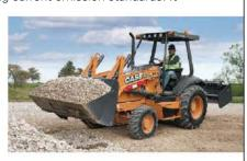
Control. The three-point hitch with variable-flow hydraulics delivers greater precision and lift capacities. An optional hydraulic power takeoff and dual tilt on the box blade provide more versatility and ditching capabilities. Its operating weight is 12,898 lbs., bucket breakout force is 9,271 lbs. and hinge pin height is 11 ft., 3 in. The machine's front loader features an optional hydraulic quick coupler to easily connect and disengage buckets and other attachments. *CaseCE.com*
