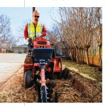
faster. A special trail wheel supports the oscillating tracks to help reduce breakover and increase stability over uneven and rough terrain; tracks "walk" or oscillate 12° for extra stability. Its trenching capacity is 48 in. deep and 8 in. wide, and easy hand controls are grouped conveniently at the operator's station. The optional backfill blade, available only from the Ditch Witch organization, eliminates the need for shovels and manual labor. *DitchWitch.com*
