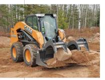
catalyst. Operator visibility and comfort, climate management and operator controls define the Case Alpha Series machines. The skid-steer cabs, which Case says are the widest in the industry, feature ultra-narrow wire side screens that improve operator visibility. Extra glass surface gives the operator 360-degree visibility. *CaseCE.com*
