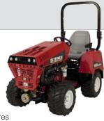
include a non-permeable, all-steel fuel tank and oversized filler neck with an EPA-approved tethered fuel cap; 200-watt halogen quartz front headlights; 1,500 psi of lift pressure, Eaton Series hydraulic pump and transmission; Peerless 2600 dual range transaxles; 5-gal. capacity hydraulic oil reservoir; 7-in. seat slides for operator fit; a new operator panel design that puts control at your fingertips; and a folding rollover protection system (ROPS) that comes standard. *SteinerTurf.com*
