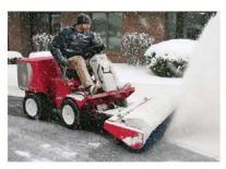
work of any clean-up job without damaging the surface below. A hydraulic cylinder angles the broom left or right from the operator's seat. Adjustable gauge wheels set the height of work for precise adjustment. Optional outrigger wheels allow for controlled adjustment when de-thatching turf. An optional front debris curtain is available for less overthrow of material. *Ventrac.com*
