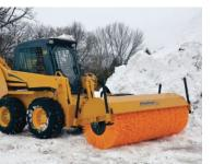
easily remove snow against curbs and walls. Skid steer models are available with 60-, 72- and 84-in. broom widths. They include a universal coupler for attaching to equipment with various hydraulic flow ratings and can be hydraulically angled 30° left or right. The PTO-driven tractor model is designed for machines with at least 30 hp. *ProTechCorp.com*
