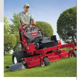
work of larger properties. All models are equipped with a 7-guage-steel, Turbo Force cutting deck, which produces the quality after-cut appearance even when mowing long, wet grass. Select models include an adjustable baffle, which allows contractors to fine-tune cutting performance. *Toro.com/professional*
