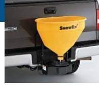
hopper. The pocket-sized wireless remote controls the rate of the two-speed spinner and toggles the electric motor on and off. The SR-210 (pictured) spreads up to a 25-ft. range and features a vertical high-flow auger that works in conjunction with the spinner; the SR-110 spreads material up to a 20-ft. range and uses a gate feed system, allowing it to handle small calcium chloride pellets or bagged ice melters. *TrynexFactory.com*
