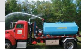
tion, irrigation of roadside vegetation, and light fire suppression. The tank is available in 1,250-, 2,000-, 3,000- and 4,000-gal. capacities, pumping up to 325 gallons per minute. It can be equipped with 3-in. grooved nozzles, side spray nozzles, and even a water cannon. All function can be controlled from the driver's seat. *AmplirollUSA.com*
