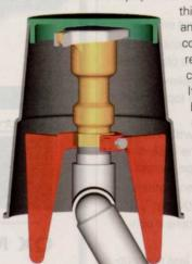
this hazard, the Claw acts like an anchor, holding the guick coupler securely in place, restraining rotational, vertical and horizontal motion. It fits inside most valve boxes without any cutting or alterations, and attaches directly to the base of the quick coupler valve with a hexagonal receptacle and single stainless steel bolt. www.underhill.us or 866/UNDERHILL
