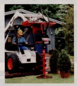
the Series 16 balances smaller flow volumes in proportion to auger diameters. The result is a cleaner hole with less loose soil and debris. For higher-capacity drilling, the Series 24 operates in a 15- to 25-gpm hydraulic flow range and delivers a maximum drilling torque of 2,018 ft.-lbs. at 2,500 psi. www.generalequip.com or 877/DIGGER-5
