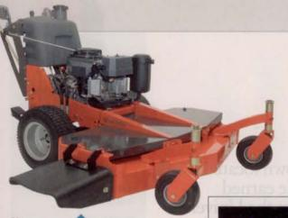
multitude of handling options. An electronic Sensor-Grip operator presence system detects the operator's hands on the handlebars. This anti-fatigue safety system requires no additional pressure to operate the mower, and it works by detecting moisture from the hands of the operator — with or without gloves on.
