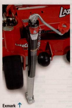
New jack (Part No. 116-1351) and receiver (Part No. 116-1049) accessories for Exmark Next Lazer Z zero-turn riding mowers allow for quick, easy access to the underside of the cutting deck — thus reducing the time and effort required to perform minor maintenance. The receiver features an easy-to-install, two-bolt construction that mounts to the mower frame without interfering with other accessories. The jack has a hassle-free crank lift design. www.exmark.com or 402/223-6300
