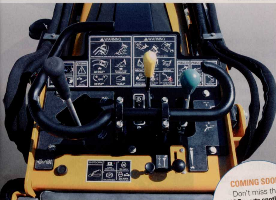
The handgrip controls on this Vermeer S400TX offers operator ergonomics.
