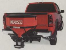
With its 400-lb. (6-cu.-ft.) capacity and lowprofile design, the new TGS 600 Tailgate Spreader from The Boss Snowplow fits Class 3 and 4 receiver hitches, and mounts/dismounts easily, saving valuable time. It also features an adjustable feed gate; adjustable material deflector; 12-in. poly spinner; an in-
